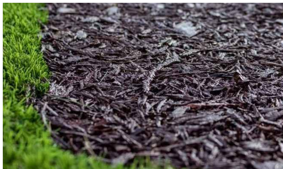
Resin bonded recycled rubber mulch safety surfacing
